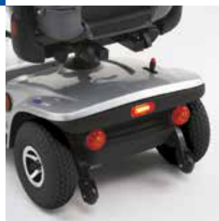
Brake light Rear brake lighting warns other people that the scooter is slowing down, thus preventing collisions.
