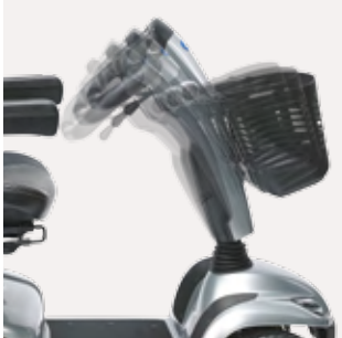
Finite tiller movement Individuals can easily adjust the tiller to suit their needs.
